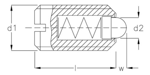
$\begin{array}{ll} d1 & = M10 \\ d2 & = 4.5 \\ Length I & = 19 \\ Spring pressure N bottom = 54.0 \\ Spring pressure N top & = 20.0 \\ W & = 2.5 \end{array}$
